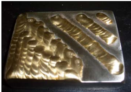
Front view of sample weld by MAGNA 28 on stainless steel
