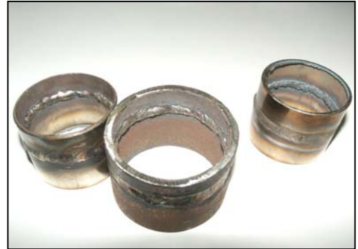
Left: Cross-sections of stainless steel pipe (2mm thick, dia. 50mm) & mild steel pipe (4mm thick, dia. 60mm), welded with MAGNA 39 showing smooth uniform bead on both sides; Right: Oxidized inside of pass welded with an ordinary solid wire.
