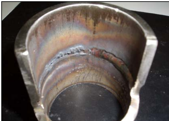
A closer view of the backside of the sample welded by Magna 39 (right), ordinary weld, (left) – rough finish exposed to oxidation
