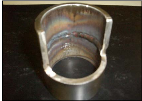
Backside of sample pipeline welded by Magna 39 (right), ordinary weld, (left) – rough finish exposed to oxidation
